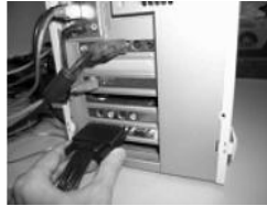
Fig. 2—2 Connection of the interface cable
