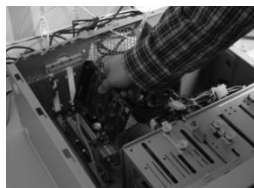
Fig. 2—1 Installation of video capture cards
