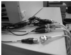
Fig. 2—3 Connecting video cameras to the BNC connectors
