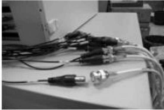
Fig. 2-3 Connecting video cameras to the BNC connectors
